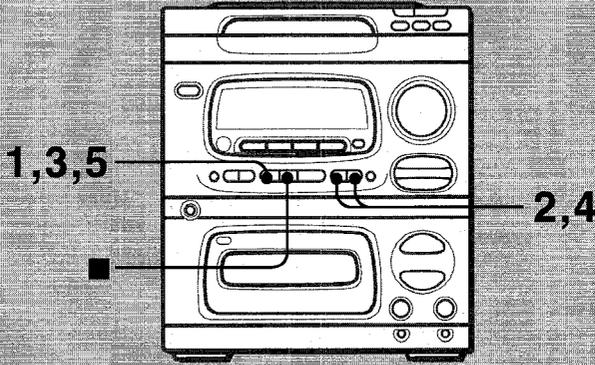
When you first connect the AC cord, the **||** SET button flashes to inform you that the current time needs to be set. Set the time as follows, while the power is still off.
