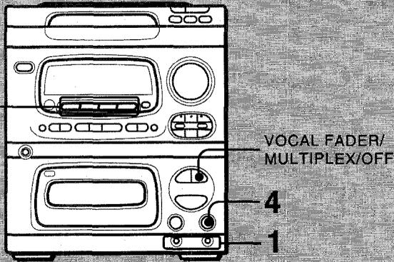
Up to two microphones can be connected to this unit, allowing you to sing along to music sources.
