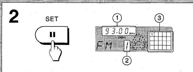
The unit can store a total of 32 preset stations. When you store a station, a preset number is assigned to the station. Use the preset number to tune in to a preset station directly. (See page 46.)
